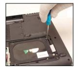
6. If there is a tab on the existing hard drive, gently pull it up and then to the outside to remove the hard drive from the bay.
